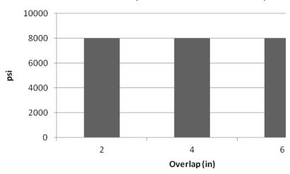
Using a contact adhesive to adhere the seam, the K-FLEX Clad® failed before the seam did. All configurations tested the same.
