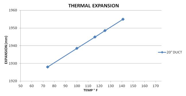
Coefficient of linear expansion = .00021%/°F (circumference of large ID (20") elastomeric duct) % expansion with a 40°F temperature change = 0.85%
