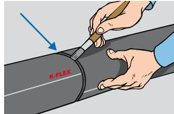
Adjacent sections of insulation should be glued at their respective ends.
