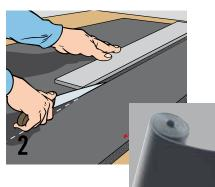
Mark the measurements of the surfaces to be insulated on the sheet and cut the required size out of the roll. **See Cutting Instructions.**
