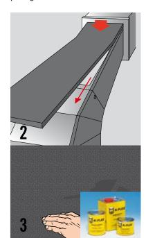
Position the uncovered edge at the starting point. Pull the backing paper off gradually, pressing the material down evenly as you go.
