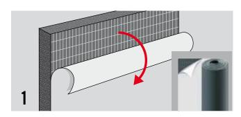
Using self-adhesive sheets, carry out the same cleaning and cutting procedures as indicated for standard sheets. The backing paper must be removed from the adhesive side before sticking it to the conduit surface. Start by pinching the foam and peeling back liner 1-2".
