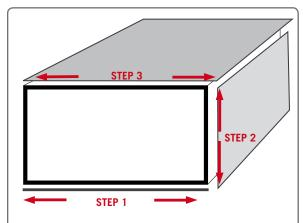
**STEP 1:** Cut the bottom piece first, making it flush with the edge.
