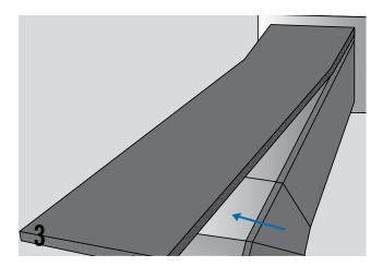
Apply K-FLEX® Contact Adhesive to the surface that has to adhere to the conduit and to the conduit surface.
